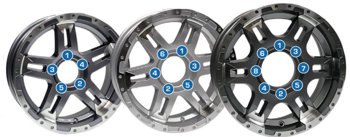
Lug Nut Installation Sequence(s)
